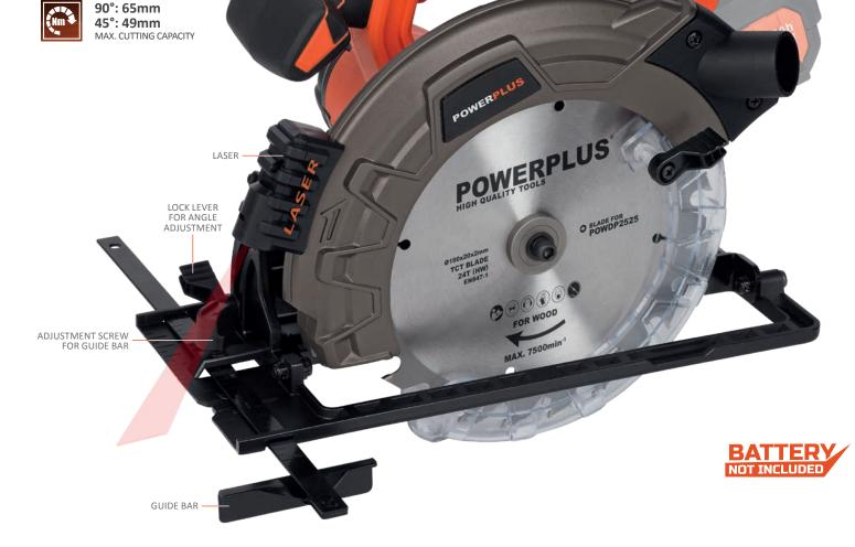
This 40V cordless circular saw has a saw blade of  $\emptyset$ 190mm that rotates at a speed of 4000min<sup>-1</sup>. You can use it to cut straight lines with the support of the guide bar or to saw mitre cuts as it also has an angle adjustment for angles between 0° and 45°. The blade can be set to the required depth. The POWDP2525 can cut up to 65mm (or 49mm at 45°). A built-in high precision laser guarantees correct, clean and accurate cuts. The worklight illuminates your workpiece.
